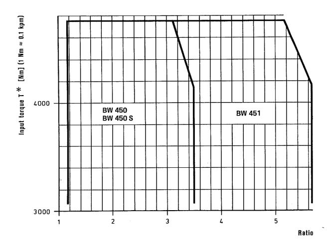
The maximum permissible gearbox input torque is plotted against the gearbox ratios. Engine outputs and speeds at continuous rating A according to DIN 6270 are taken as reference values, 10 % overload is allowed. The values are applicable to both rotational directions of the output shaft "enginewise" and "counter-enginewise" rotation. Max. permissible input speed (at continuous rating A) is 2000/min. Permitted engine idling speed < 800/min, please indicate on order sheet.
